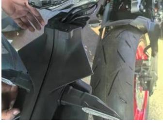
4. Remove the 6 screws from the plastic license plate frame. As the picture shows:
