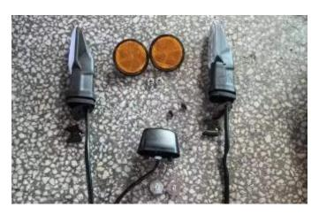
7. Mount the 3 lights on the iron license plate mounting bracket and add 2 aluminum posts to the rear license plate light location. As the picture shows:
